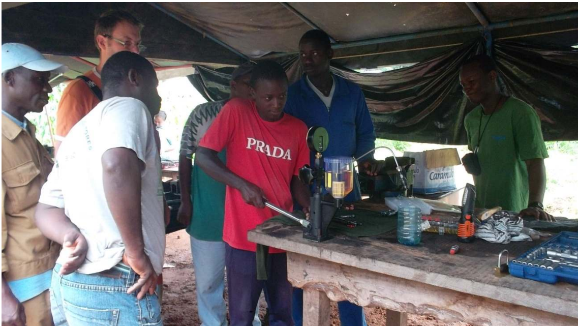
... where the participants also tried to test the injector opening pressure.
