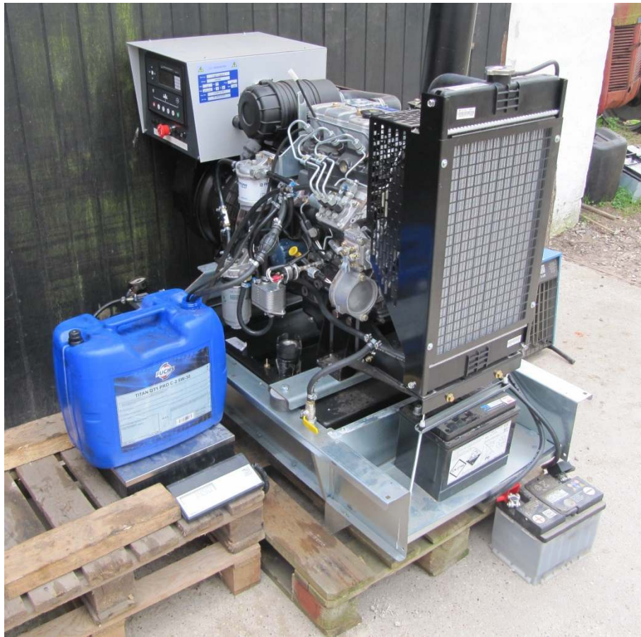
The fuel consumption was measured by weighing the fuel tank on a digital balance.
