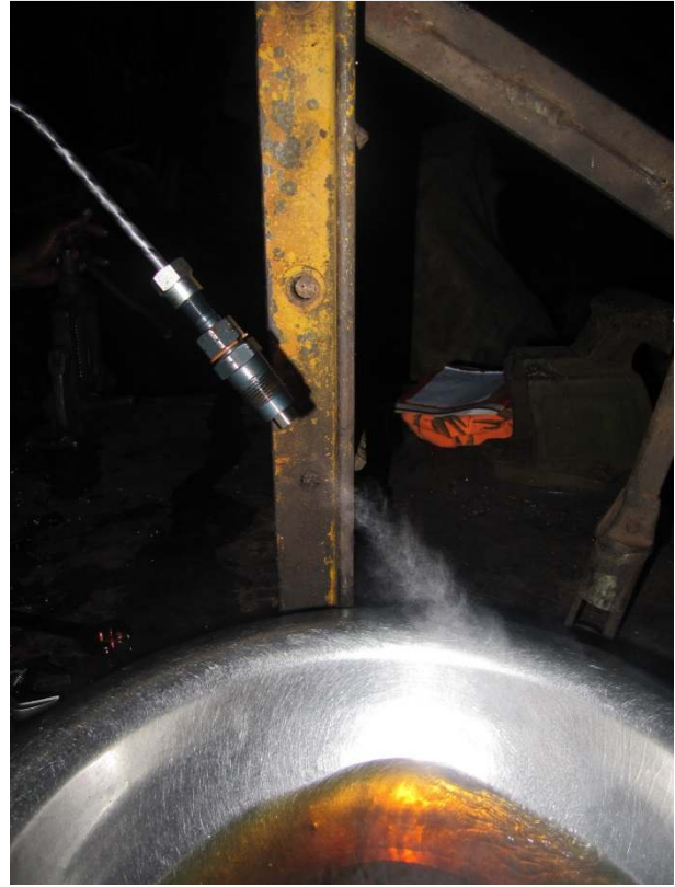
The adjustment of the injector spring(left) and the test of the spray and opening pressure(right)
