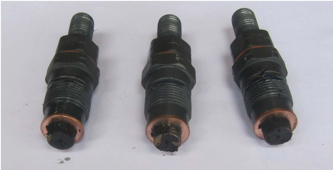
The original injectors after just 1 cold start and approximately 1h operation on PPO.
