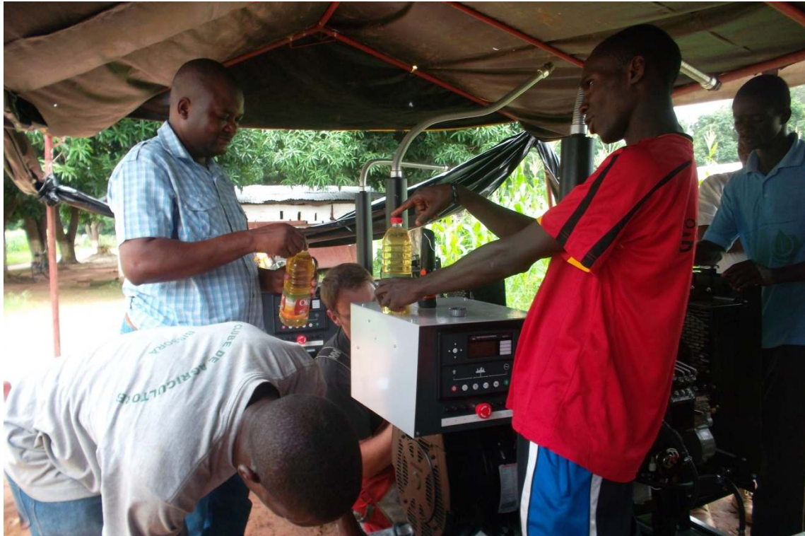
Test run after the 1 st conversion with refined cooking oil from the shop.
