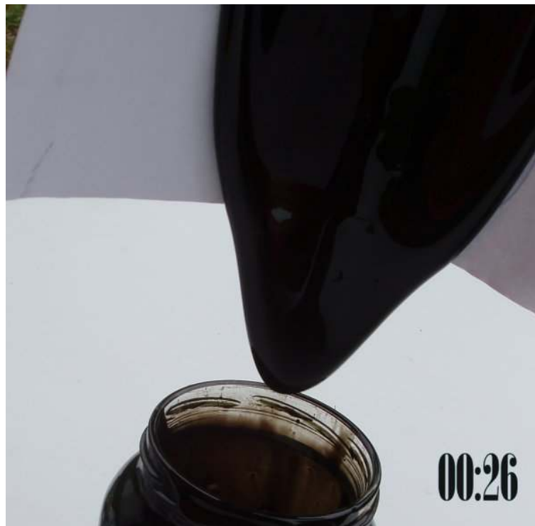
The photo shows polymerized lube oil with very high viscosity, taken out from an engine, which didn't have the lube oil changed in time. To illustrate the high viscosity, the lube oil was poured out on a piece of A4 paper,
