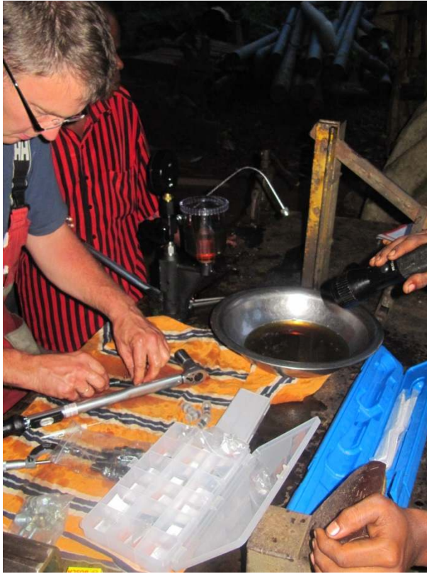
The adjustment of the injector spring(left) and the test of the spray and opening pressure(right)
