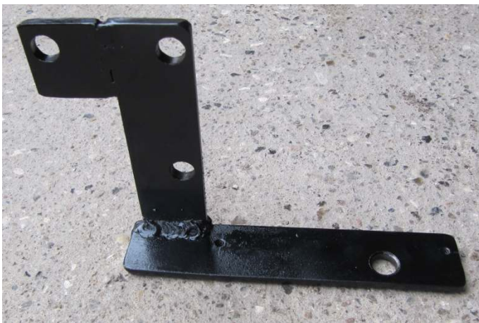
(Left)Special bracket designed for holding the heat fuel exchanger. (Right) Heat exchanger and bracket being installed on the genset.
