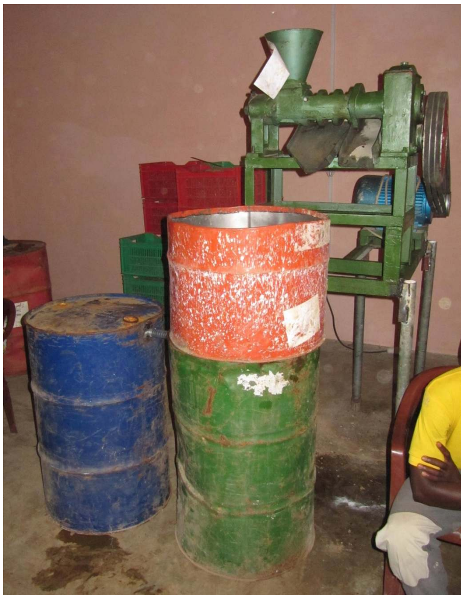
The oil expeller installed on legs, and preparing the 3-stage sedimentation system, using oil drums.
