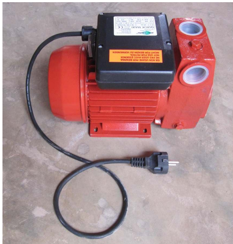
2 units Sealand(Italy) Impeller pumps, 230V, 590W(0,8hp) max. 40-50liter/min, max pressure 2,5bars (25m), Self priming.
