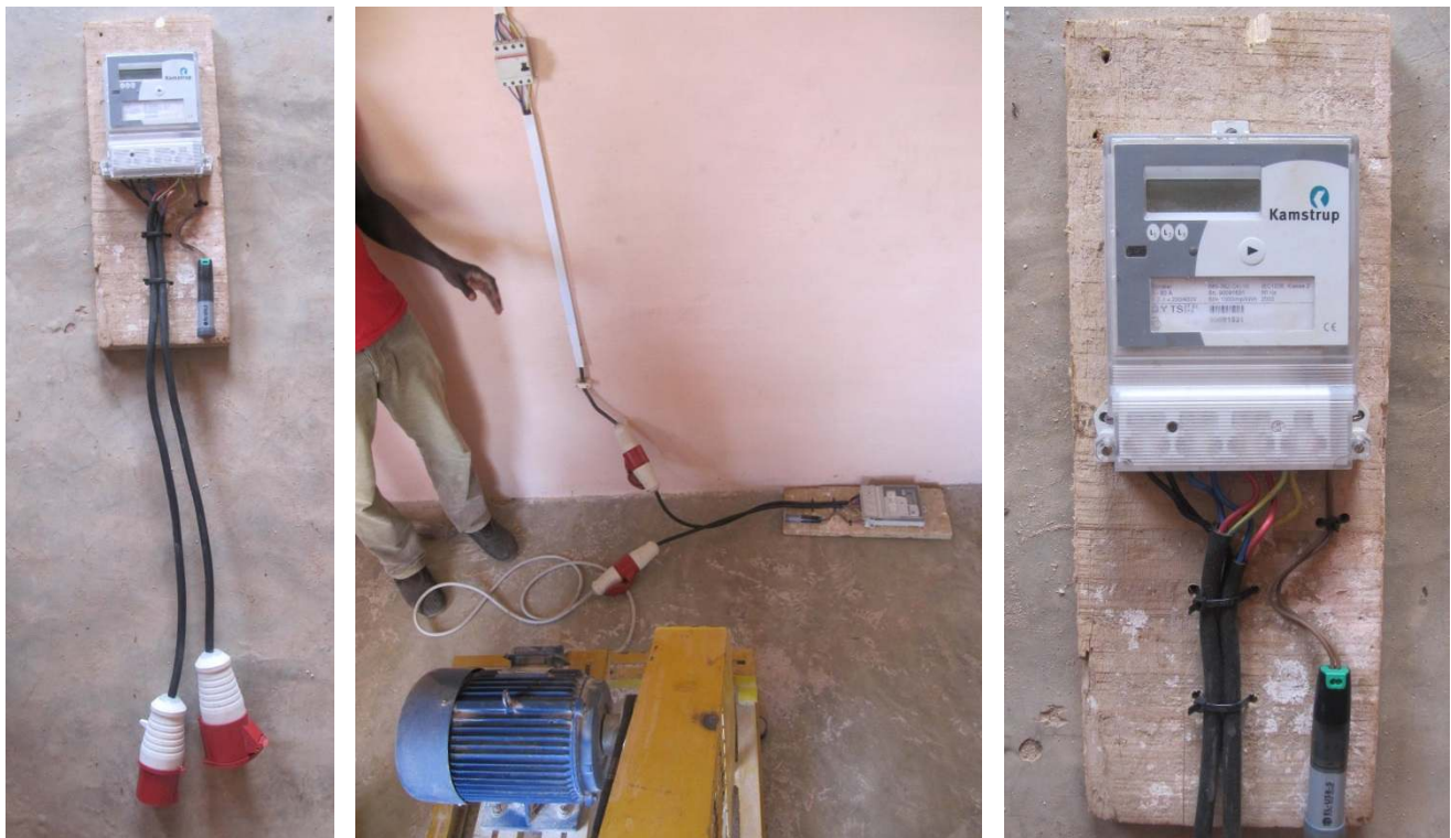
Left photo: The meter with cables, socket and plug, and data logger. Middle photo: The meter installed on the power supply for the maize mill. Right photo: Detail of the meter and USB data logger.
