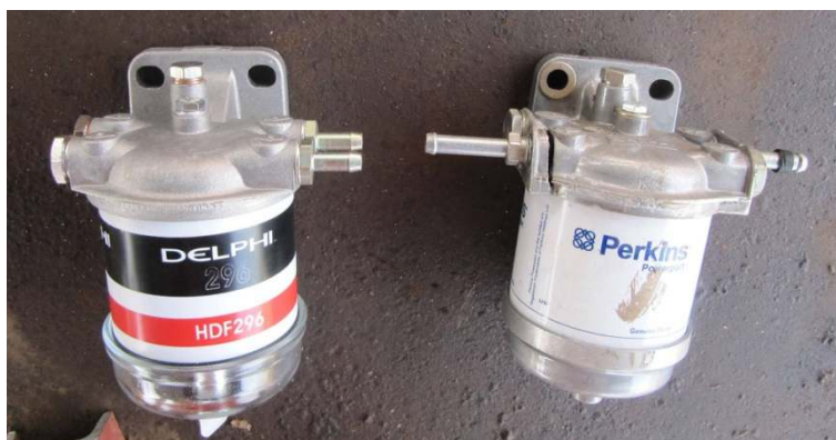
Fuel filter to replace original filter on the genset, which was broking during august workshop.
