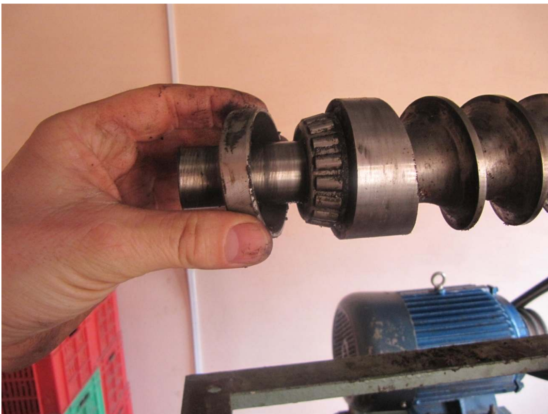
During test of the oil expeller the main bearing for the screw broke. I new bearing was found on the local market and changed.
