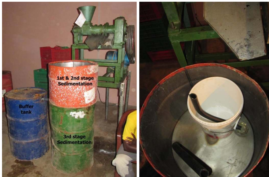
3 stage sedimentation system and buffer tank(left). Detail of 1 st & 2 nd stage sedimentation system(right)
