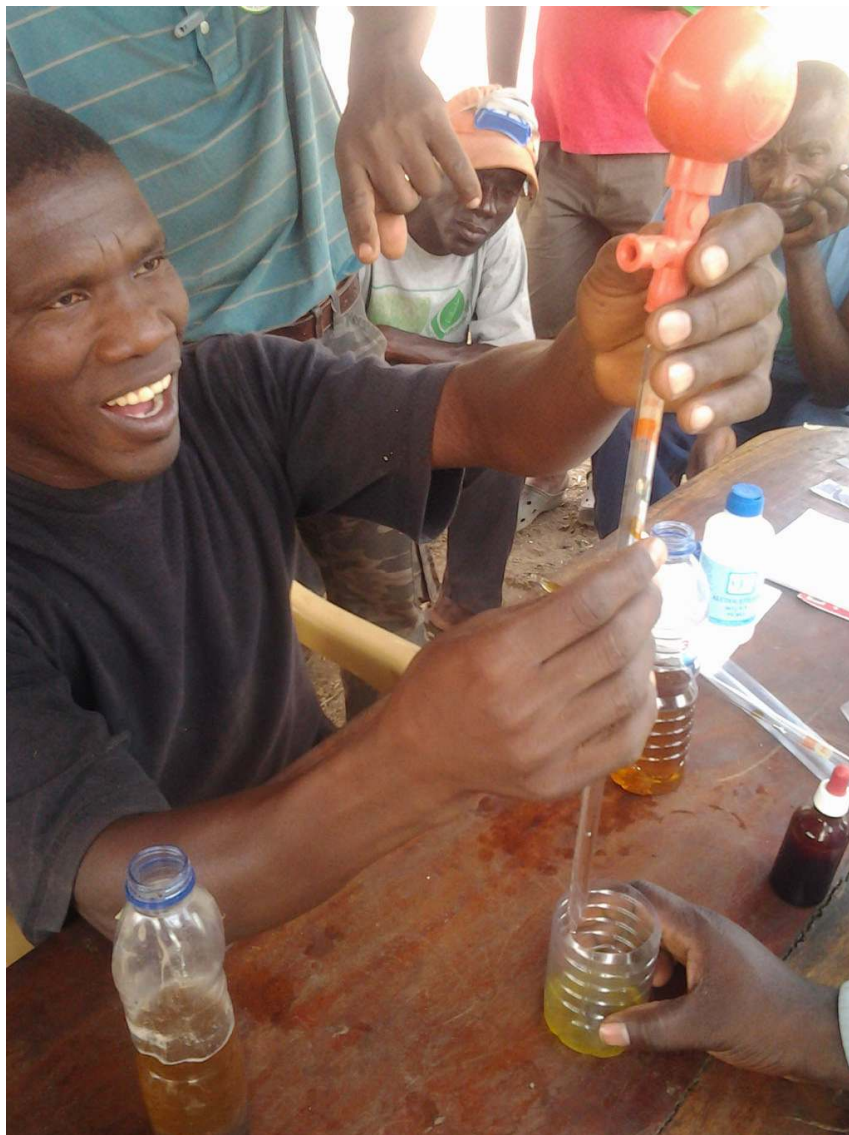
Testing the acidity of the PPO (FFA)
