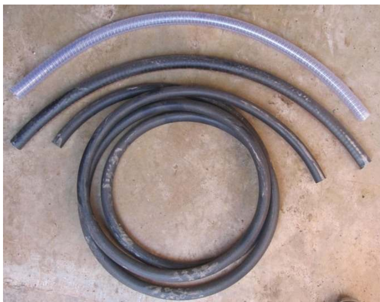
Fuel hoses to connect pumps and filters
