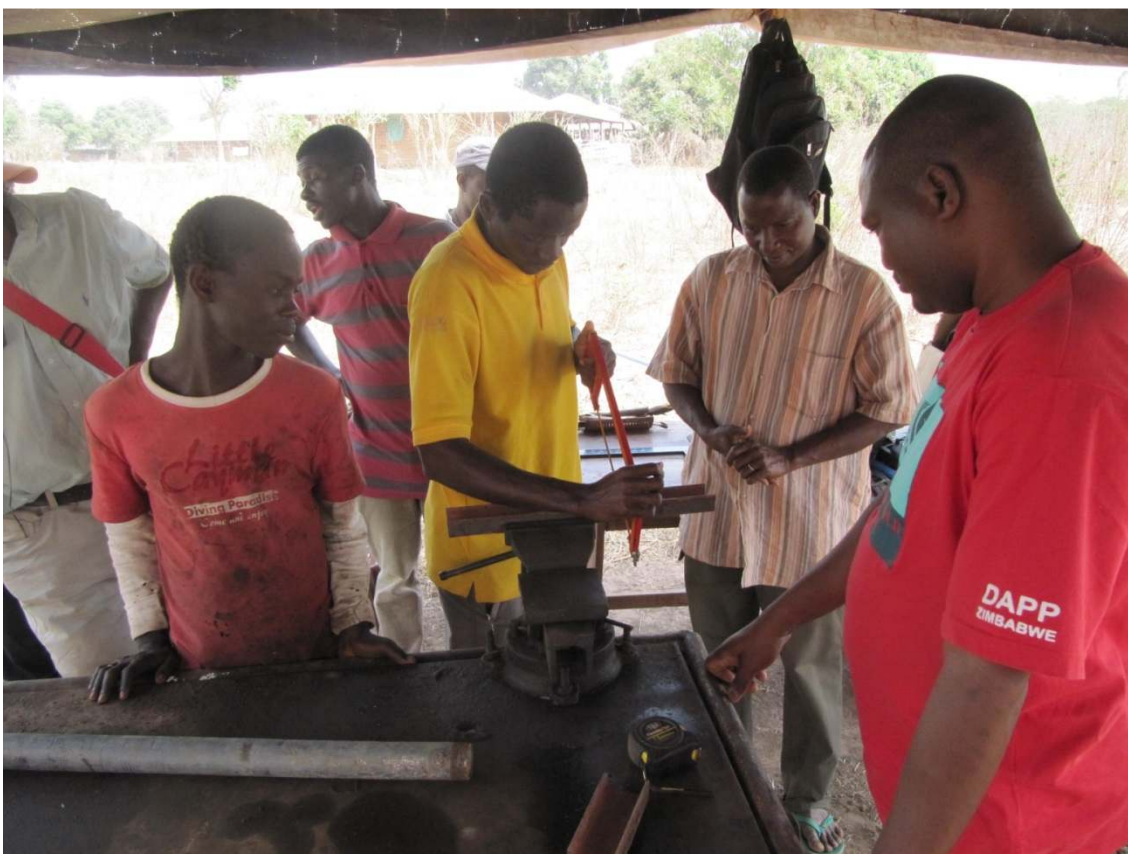
Preparing steel parts for frame and legs to support the oil expeller.
