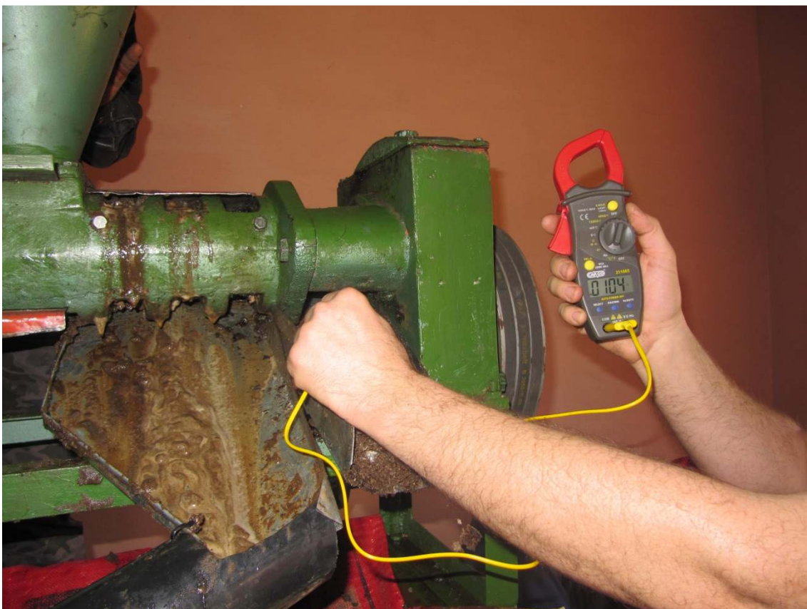
Measuring temperature of the oil and press cake released from the oil expeller – here press cake temperature 104°C.
