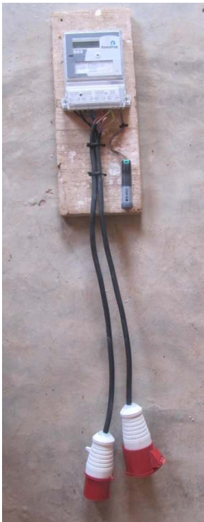
Left photo: The meter with cables, socket and plug, and data logger. Middle photo: The meter installed on the power supply for the maize mill. Right photo: Detail of the meter and USB data logger.
