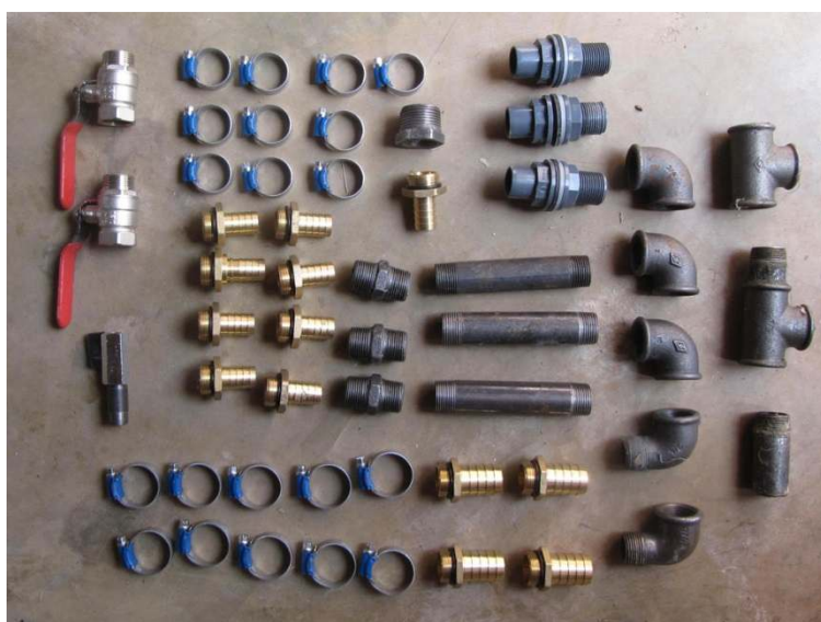
Pipe fittings to connect filters and pump.
