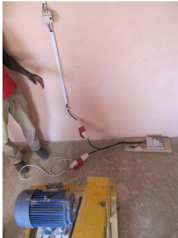
Left photo: The meter with cables, socket and plug, and data logger. Middle photo: The meter installed on the power supply for the maize mill. Right photo: Detail of the meter and USB data logger.
