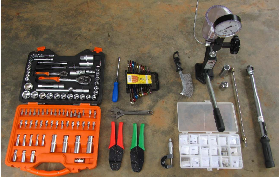
The special tools for the conversion workshop. Including injector tester, torque wrench, adjustment shims and micro meter, crimping tools, Socket set etc.
