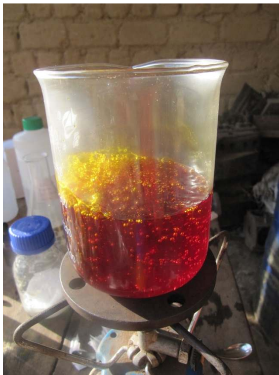
Water evaporation from palm oil in Gamena
