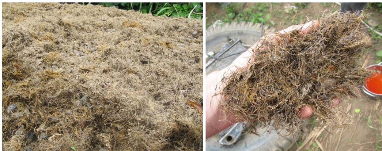
Dried fibers from the palm fruits could be used as insulation for the process tank.
