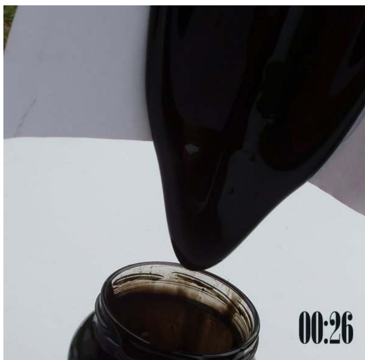
The photo shows polymerized lube oil with very high viscosity, taken out from an engine, which didn't have the
