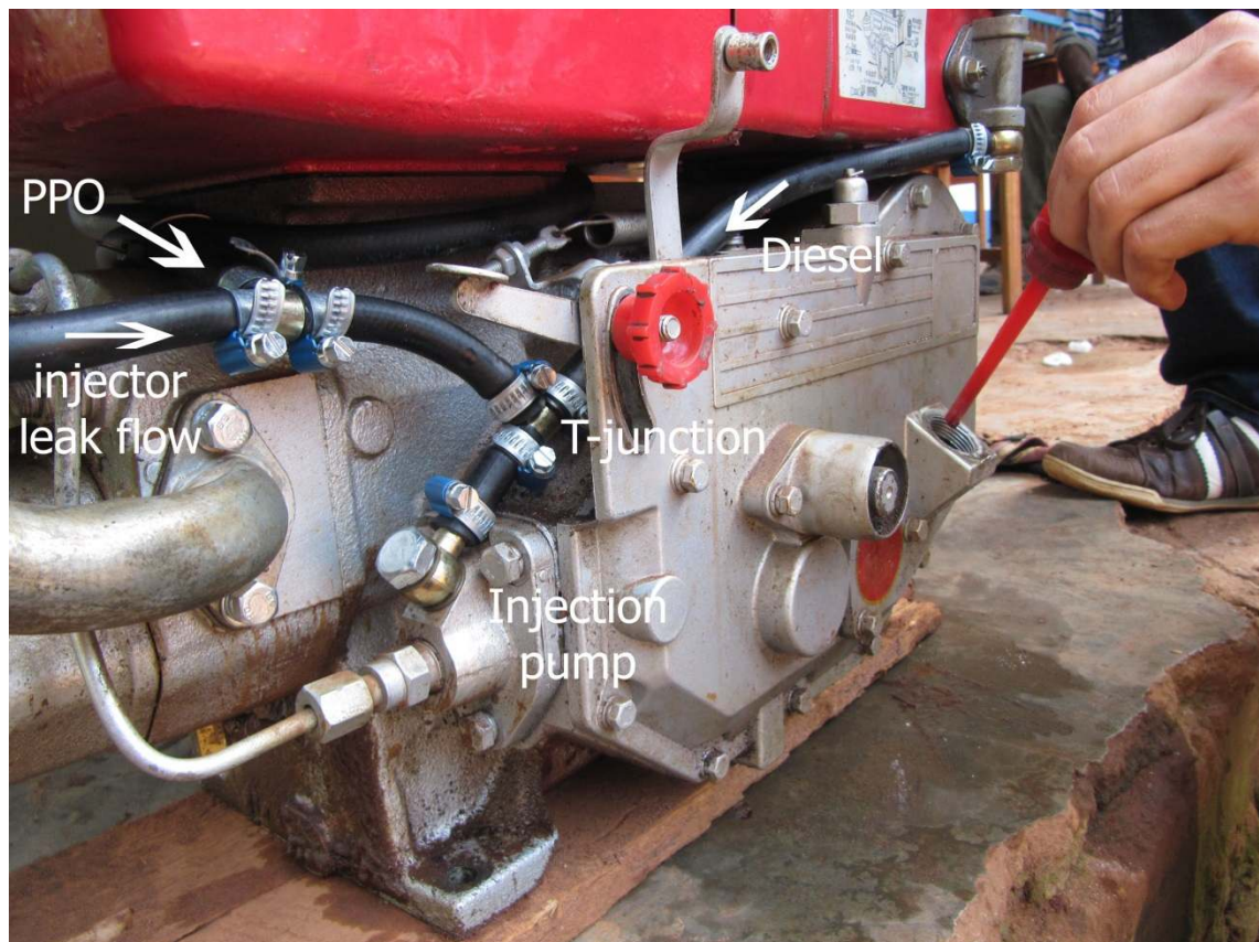
Fuel cycle for the Poussa 2-tank system.
