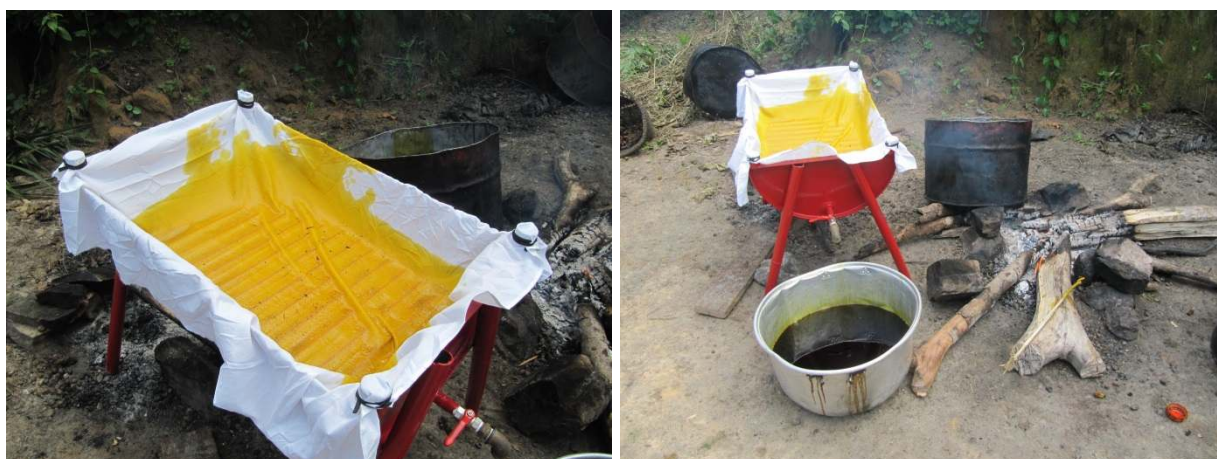
An initial rough filtration using a filter membrane attached to a half cut oil drum.
