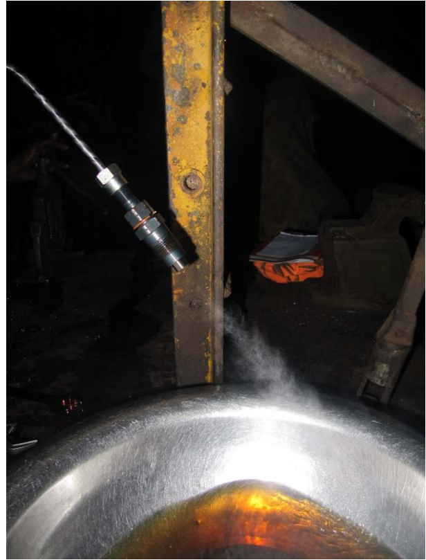
The adjustment of the injector spring(left) and the test of the opening pressure(right)
