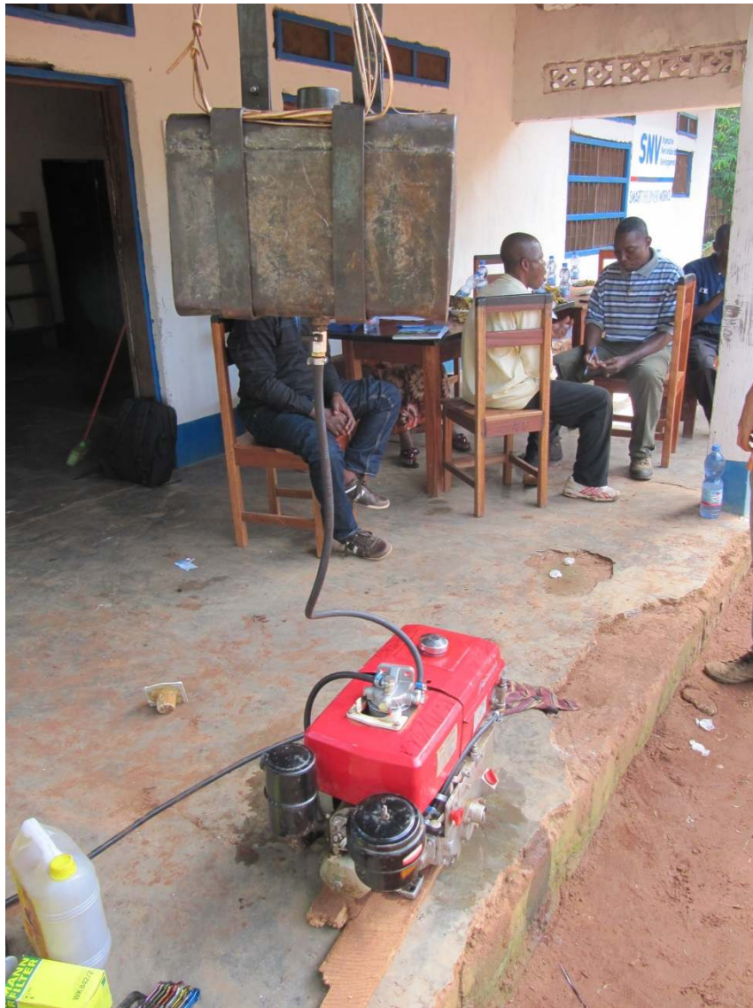
The PPO tank elevated approximately 1 meter above the engine.
