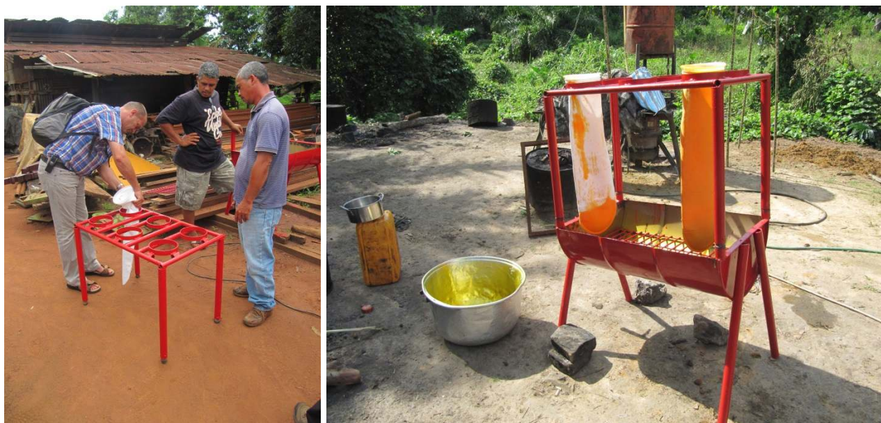
A finer filtration using filter bags hanging in a support frame, designed for the purpose.
